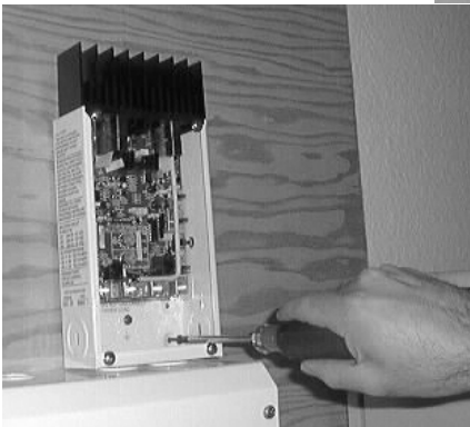
Figure 2-3 Mounting the C-Series Multifunction DC Controller
