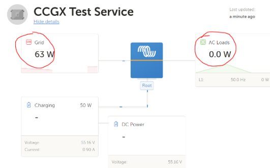
Picture right showing 0.0W AC Loads and 63W consumed power from the grid. In reality a 600W load is connected.
