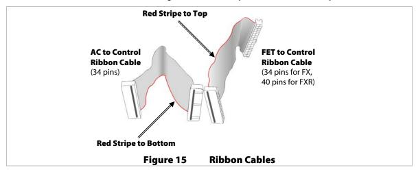
8. Install the ribbon cable that is bent on one end to the FET PCBA and the Control PCBA. (See Figure 16 and also Figure 7 if necessary.) In the FX inverter, this cable has 34 pins. In the FXR inverter, it has 40 pins. Make sure the red stripe is oriented toward the **top** of the chassis. Push down on each end until the levers click and the plug is secure.
