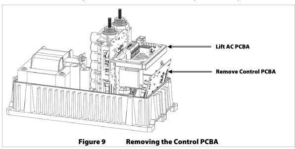
14. Before removing the AC PCBA, using a pair of long-nose pliers, disconnect the white and black AC output wires connected at the bottom of the board. (See Figure 10 for the location of the wire connectors.) Remove the AC PCBA.
