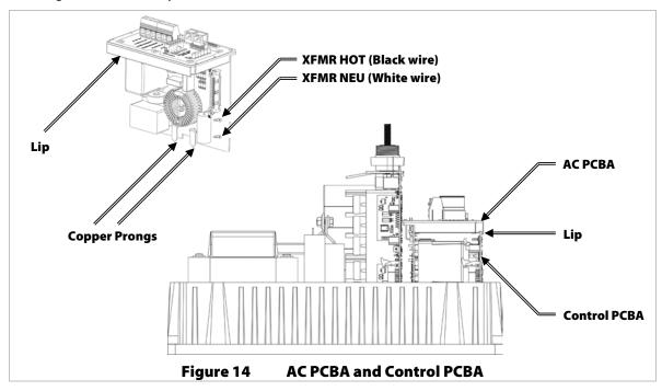
6. With the AC PCBA lifted as high as possible, guide the Control PCBA into its slot in the chassis. Lower the AC PCBA over the top of the Control PCBA. As shown in Figure 14, there is a "lip" on the AC PCBA that fits over the top of the Control PCBA.
